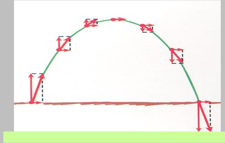
The ball has a horizontal velocity component that does not change - Similar to throwing the ball off the cliff.
